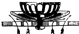
MAUDSLAY'S DISC VALVE FOR AIR PUMP. Section.
